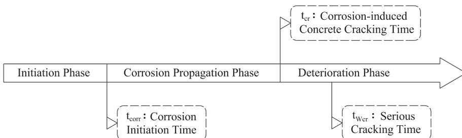
Fig. 1. Phases of chloride-induced corrosion process of reinforcing steel.
