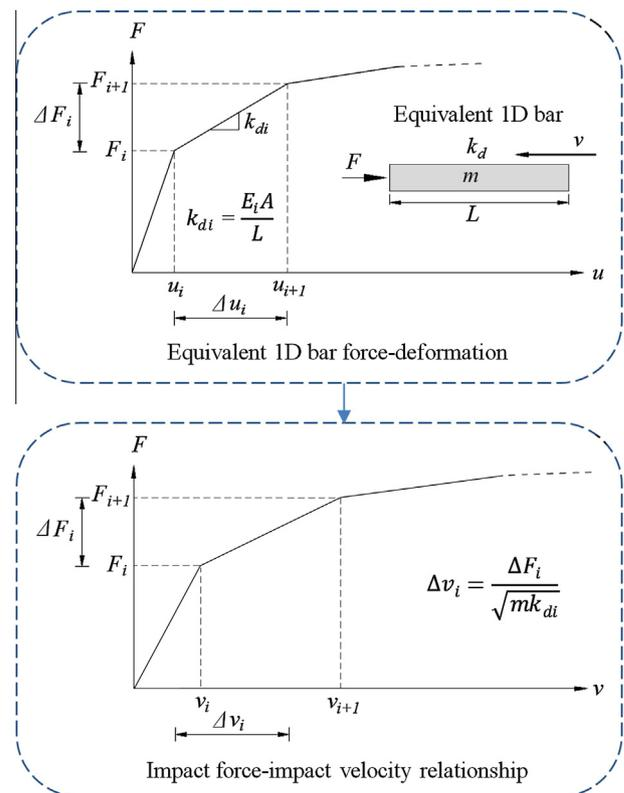
Fig. 1. Estimation of debris impact force using equivalent 1D bar model [18].
