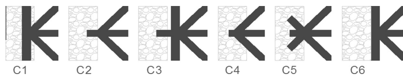
Fig. 1. Different type of wall-to-half-timbered wall connections (adapted from Cardoso [11]).
