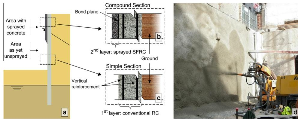
Fig. 1. Bi-layer diaphragm walls: (a) general scheme; (b) compound cross-section; (c) simple cross-section; and (d) spraying of an experimental wall.
