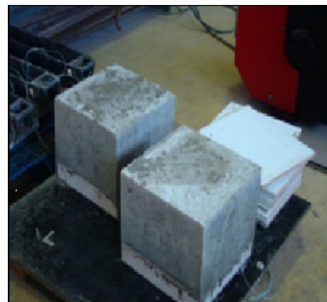
Fig. 1. Bilayer samples made of concrete and rock.
