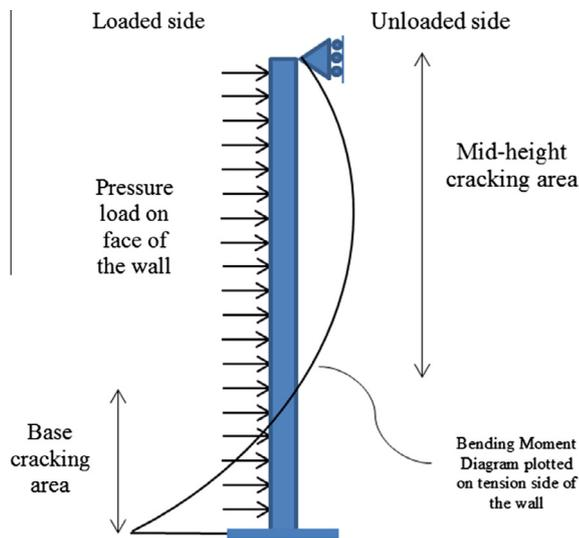
Fig. 1. Diagram for illustrating base cracking and mid-height cracking.
