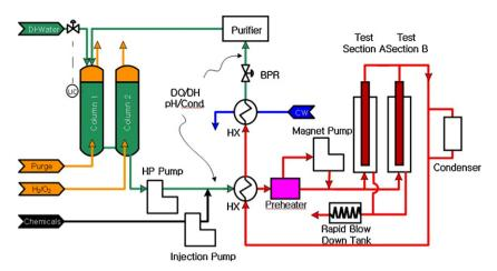
**Fig. 1.** Schematic drawing of AOA simulation test loop. A test loop was designed and used to simulate the conditions of AOA on the cladding surface. The test loop has a test section A with a low flow rate at a low temperature, and a test section B with a higher flow rate at a higher temperature, respectively. BPR = back pressure regulator; CW = cooling water; HP = high pressure; HX = heat exchanger; LIC = liquid injection controller.
