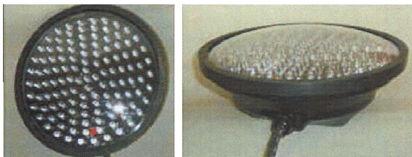
Fig. 1. Detail of the housing and the rubber joint of a traffic light of 200 mm in diameter.
