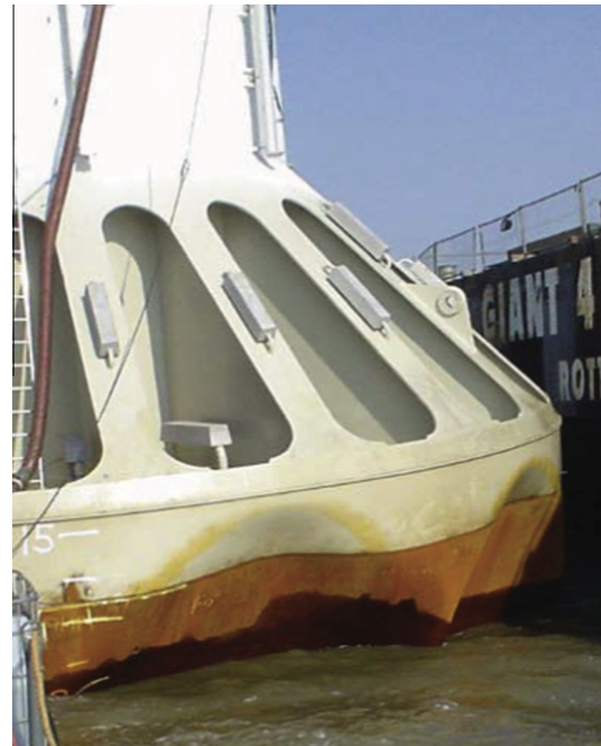
Fig. 4. Buckling failure in Wilhelmshaven 2005.
