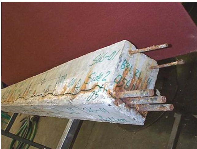
Fig. 1. Corrosion cracks on surface of concrete beam.
