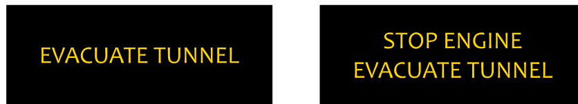
Fig. 1. Schematic representation of one of the TIS messages in the Southern Link Tunnel (left) and the Göta Tunnel (right) [translated from Swedish].
