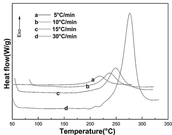
Fig. 2. DSC curves of TDE-85/BMI/BADCy copolymer at different heating rates.
