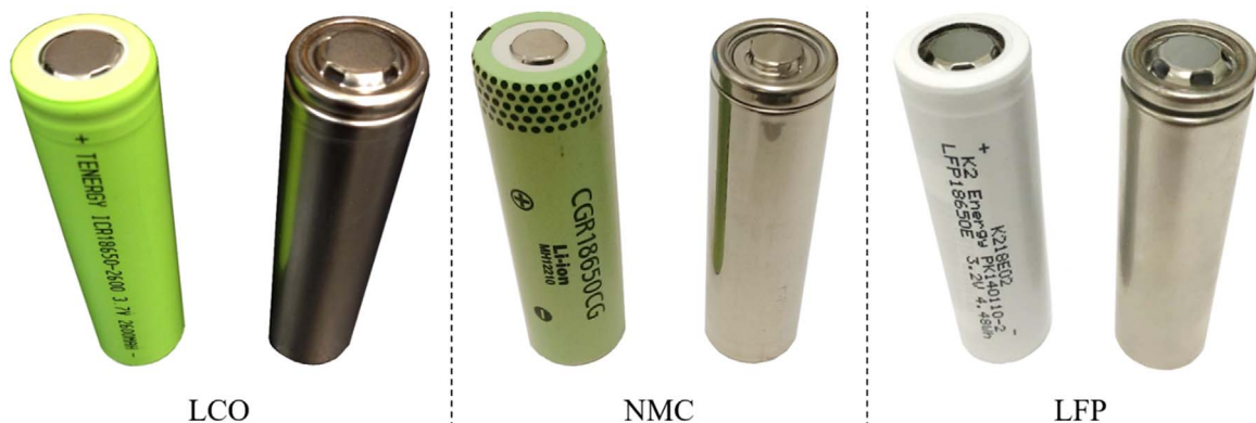
Fig. 1. Tested LIB cells with (left) and without (right) plastic packaging.
