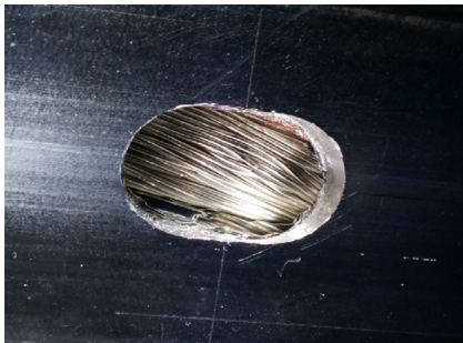
Fig. 3. Helium inlet hole drilling and wrap removal.
