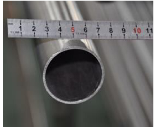
Fig. 2. TF jacket section (316LN).
