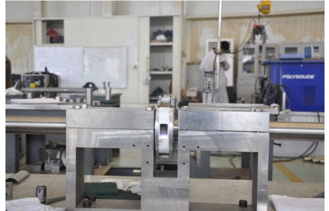
Fig. 3. The automatic welding for TF jacket.
