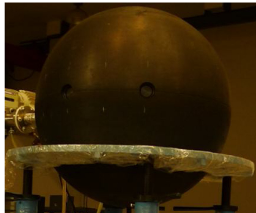
Fig. 2. Depleted uranium shell assembly.
