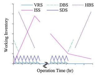
Fig. 2. Working inventory of the fuel cycle during a day.
