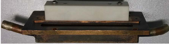
Fig. 1. Heat exchanger and ceramic.
