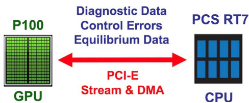
Fig. 2. The software architecture of integrating P-EFIT into PCS: PCS invokes P-EFIT directly, data is transferred between PCS and P-EFIT through PCI-E.
