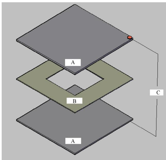
**Fig. 1.** Experimental modal (A: stainless steel sheet; B: rubber spacer; C: high-voltage source).
