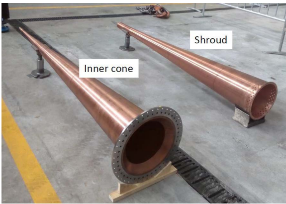
Fig. 1. Electroformed BD cone and shroud.
