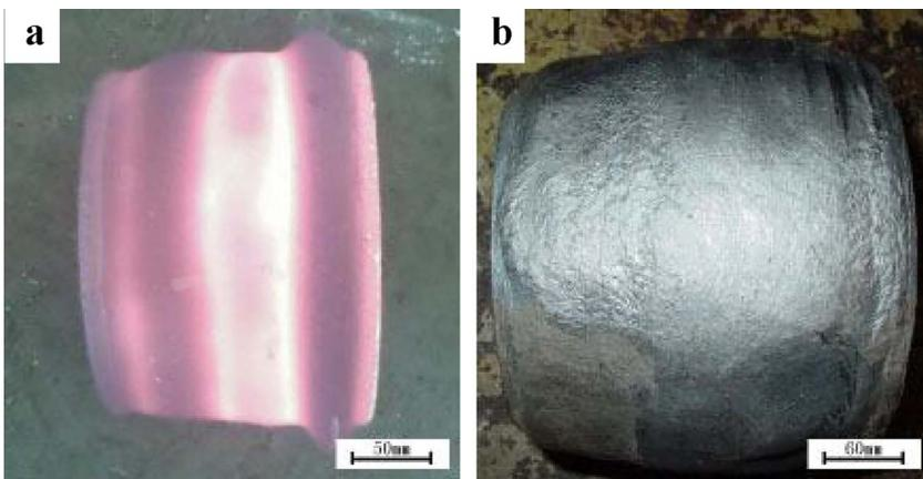
Fig. 2. Canning and forging blanks of V–5Cr–5Ti alloy after hot forging: (a) canning; (b) forging blank.
