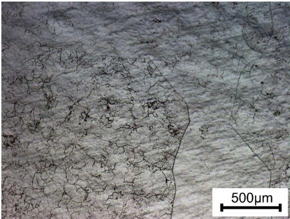
Fig. 1. As-cast microstructure of V–5Cr–5Ti alloy.
