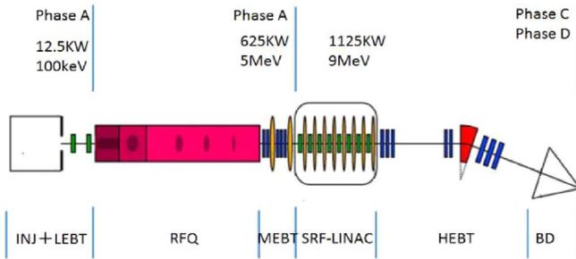
Fig. 1. Schematic view of LIPAc and commissioning Phases.
