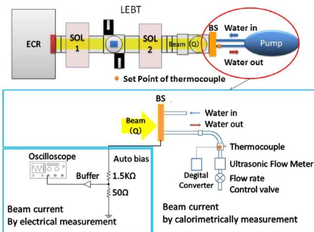
Fig. 2. Schematic view of location of TC for BS in the LEBT.
