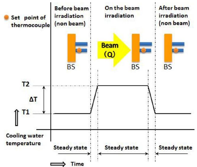
Fig. 3. Chronological change of cooling water temperature evolution by the beam irradiation.
