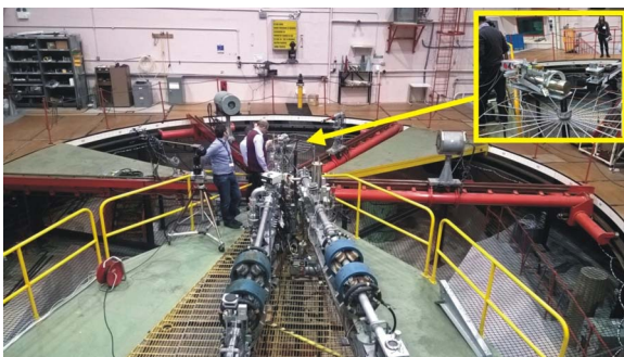
Fig. 1. Experimental hall inside the Chadwick facility. The NG is located in the centre of the hall (in the right upper corner is enlarge photo of NG). The two long counters and the NE-213 scintillator are situated above the red rails in the centre of the above image. (For interpretation of the references to colour in this figure legend, the reader is referred to the web version of this article.)
