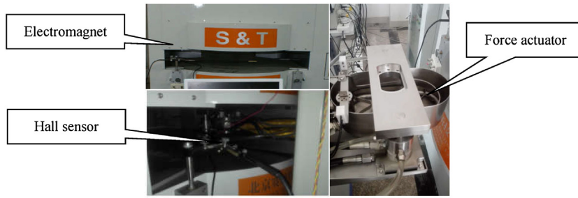
Fig. 1. Experimental system: the multi-field coupling testing device.
