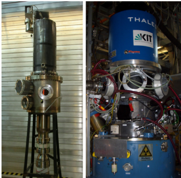
Fig. 1. EU 1 MW, 170 GHz gyrotron prototypes for ITER: short-pulse gyrotron (left) and industrial CW tube, installed with its auxiliaries in the Oxford Instruments (OI) super-conducting magnet at KIT (right).
