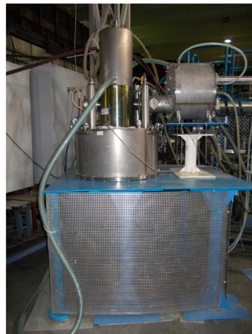
Fig. 2.1. (42 GHz Gyrotron for ECRH in SST-1).
