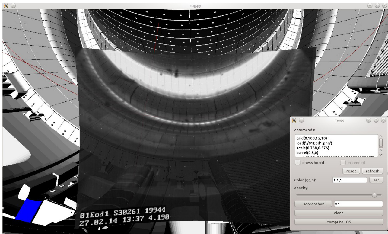
Fig. 2. Mapping a camera image into the 3D model applying geometrical adaptations (see text).
