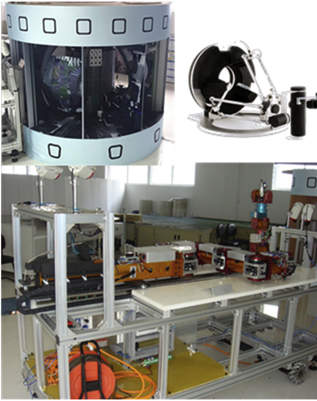
Fig. 1. Our platform: a 1/10 scale tokamak model, a haptic device Omega 7 and a remote handling manipulator.
