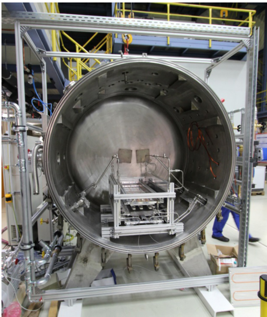
Fig. 1. Open vacuum vessel with experimental setup behind water cooled aluminum shields.
