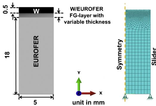
Fig. 1. The sketch and mesh of the FE model.
