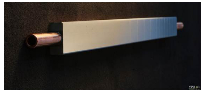
Fig. 3. Cu-PFU prototype with W coating ( \sim 30 \mu\text{m} ).
