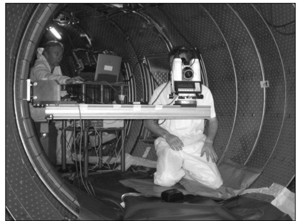
Fig. 2. Leica TM5100A Theodolite used in Tore Supra in 2000.
