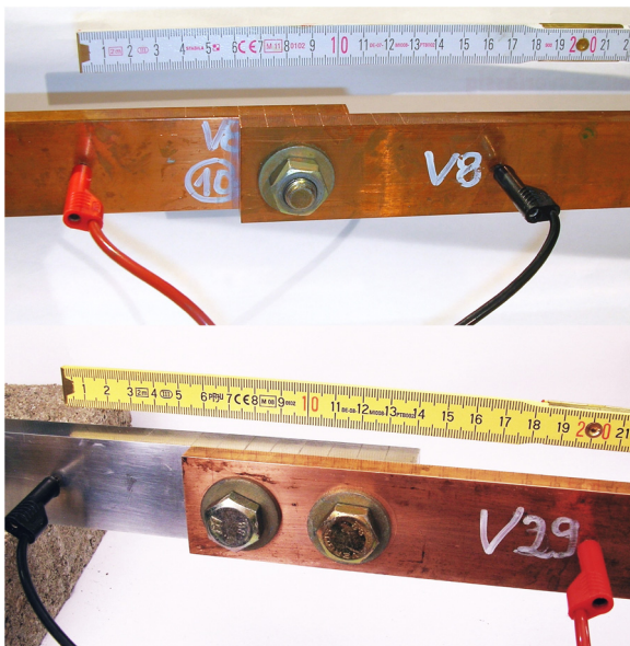
Fig. 1. Test samples, first test batch (40 mm overlap) at the top and second test batch (80 mm overlap) at the bottom.
