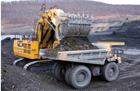
Fig. 1. High impact shovel loading operation (HISLO).
