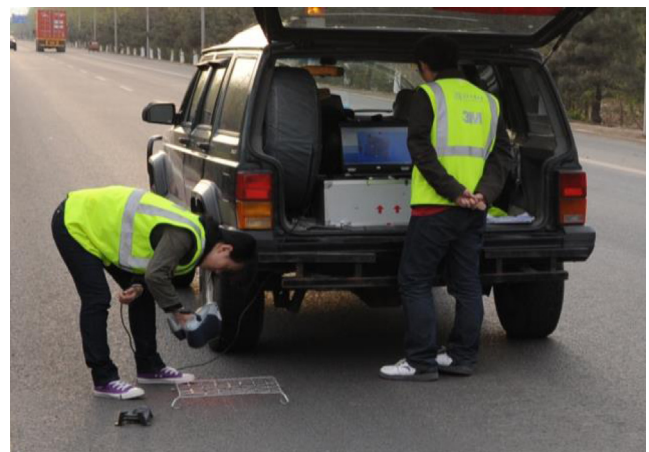
(b) Field acquisition of pavement macro texture
