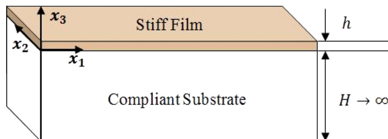
Fig. 1. Schematic of the film/substrate system.
