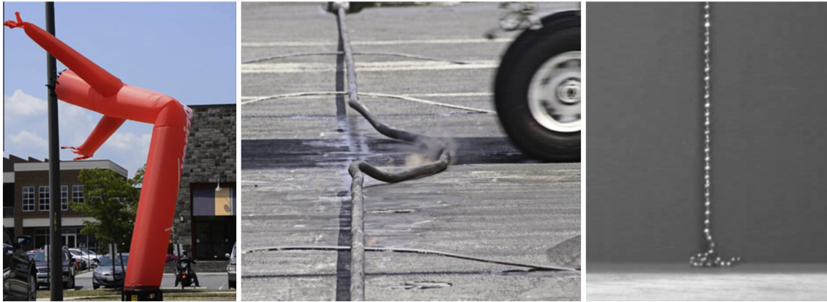
Fig. 1. Real systems with discontinuous, or approximately discontinuous, moving features. Left: A kink moving upward in a tubular Airdancer ® ( airdancers.com/about/ ) membrane (still from a film courtesy R.B. Warner). Center: A propagating impact in an aircraft arresting cable ( commons.wikimedia.org/wiki/File:AircraftCarrier3-wire.jpg ). Right: A chain falling onto a table (still from a film courtesy D. Aliaj and R.B. Warner). The table, or the pile of chain on the table, acts as a positive supply of stress (momentum) and a negative supply of power (energy).
