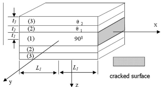
Fig. 1. Geometry of cracked element.
