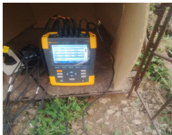
Fig. 1. The three-phase data logger connected in the case study feeder pillar.
