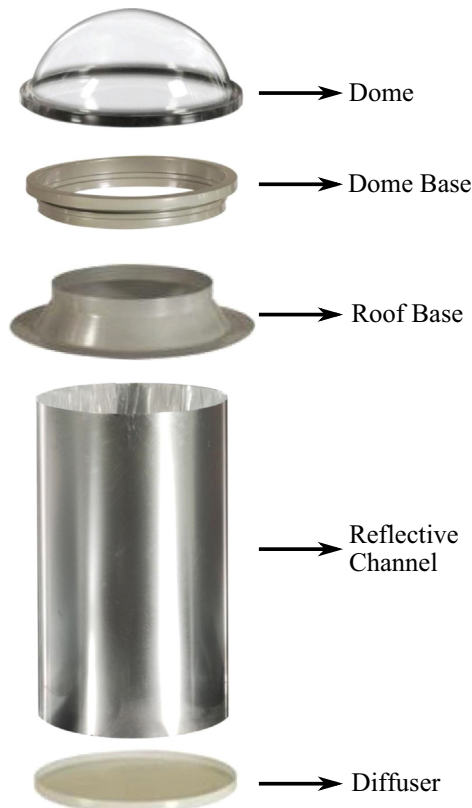
Fig. 1. Tubular daylighting device.
