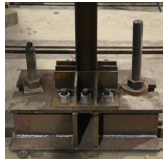
d. Column base fixture
