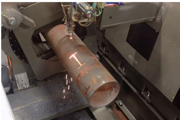
Fig. 2. Example of the laser cutting process on a CHS profile.
