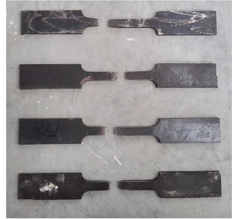
Fig. 3. Specimens of tensile testing after failure.
