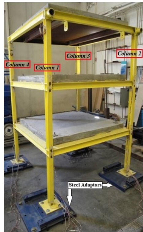
Fig. 1. Three-story steel frame structure.
