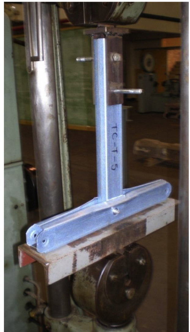
Fig. 4. Lockbolt truss connection, testing machine set-up.
