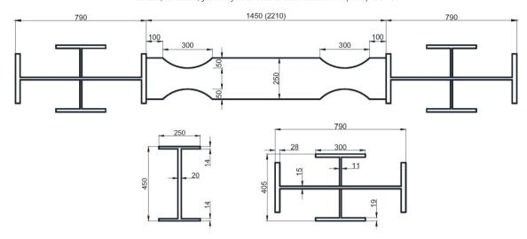
Fig. 1. Beam and columns details.
