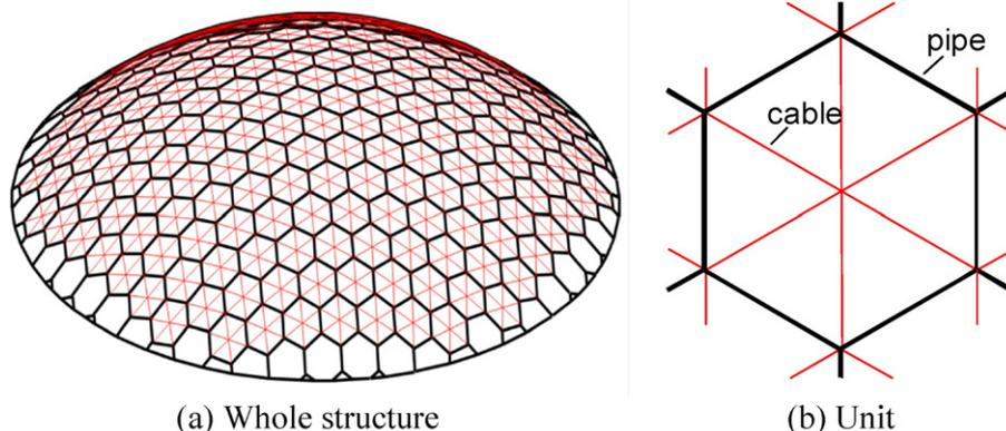
Fig. 2. Cable-stiffened single-layer latticed dome of hexagonal meshes.
