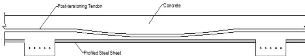
Fig. 1. Typical post-tensioned composite slab (Ranzi et al. [5,6]).
