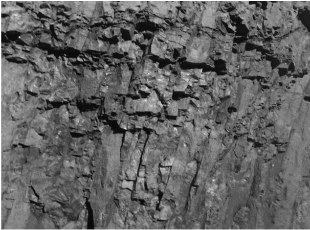
Fig. 1. Exposed columnar jointed basalt in the diversion tunnel of Baihetan hydropower station.
